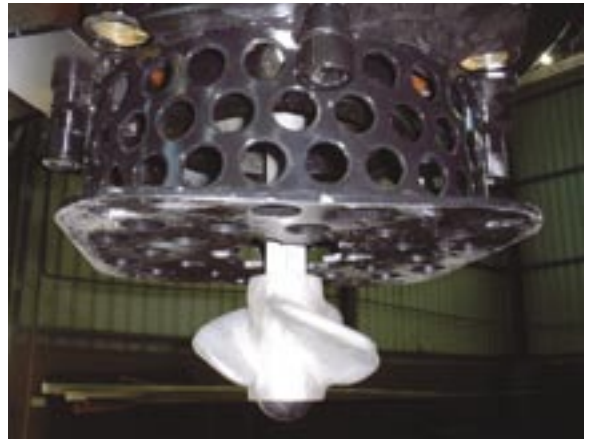
Bottom mounted HVOF coated agitator on the ITT Flygt HP 5540 centrifugal pump
