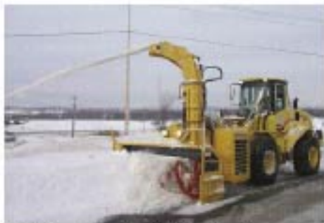
LARUE D55 detachable loader mount, mechanical drive, 300 HP, 8500 lbs, 36 in. ribbon auger, 40 in. impeller, telescopic chute
