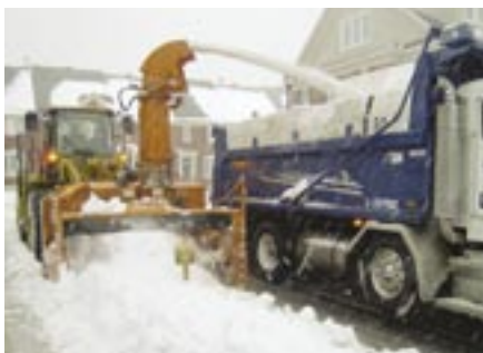
LARUE D55 Detachable snowblower mechanical drive, 275 hp, 8500 lbs, 36 in. ribbon type screw, 40 in. turbine, telescopic chute
