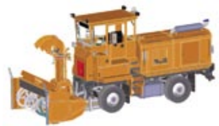
LARUE T60 R36 Self-propelled snowblower, hydrostatic drive, Cat C9 350 hp engine, 36 in. ribbon type screw, 40 in. turbine, telescopic chute
