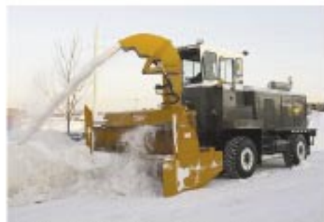
LARUE 7060 Series 226 self propelled hydrostatic drive, Detroit Diesel Series 60 533 HP engine
