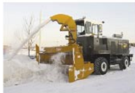
LARUE 7060 Series 226 self propelled hydrostatic drive, Detroit Diesel Series 60 533 HP engine
