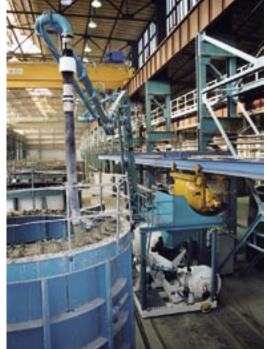
The squeeze valve on the end hose prevents the concrete from after-dripping when the boom is swivelled. The EBC control on the AUTOCOR also damps any unwanted boom vibrations and prevents the unintentional touching of floor beams and pillars in the production workshop.
