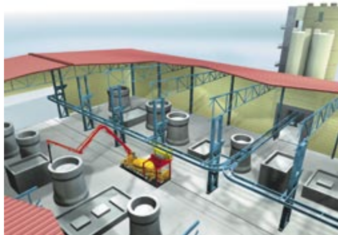
Schematic diagram of the AUTOCOR in a precasting plant. The flexible placing boom makes it possible to fill varying types of formwork.
